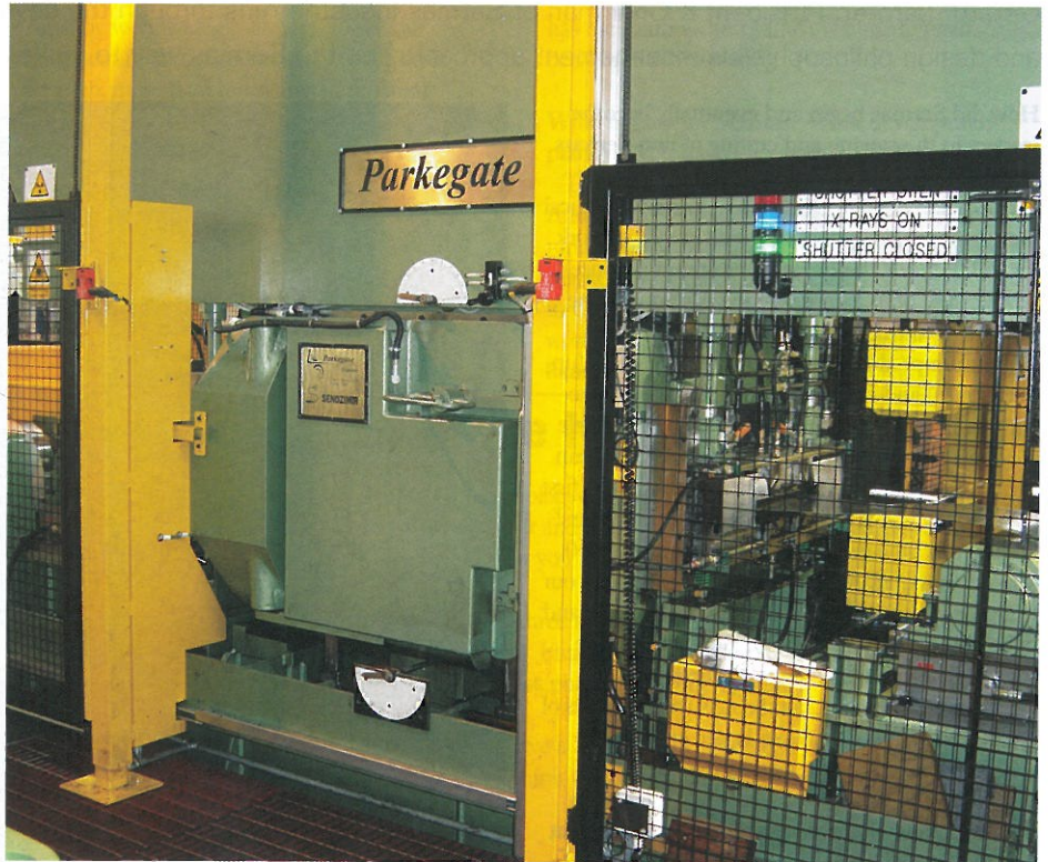
Zenzimir Mill re-engineered by Parkegate (originally at Outokumpu and now in China)
